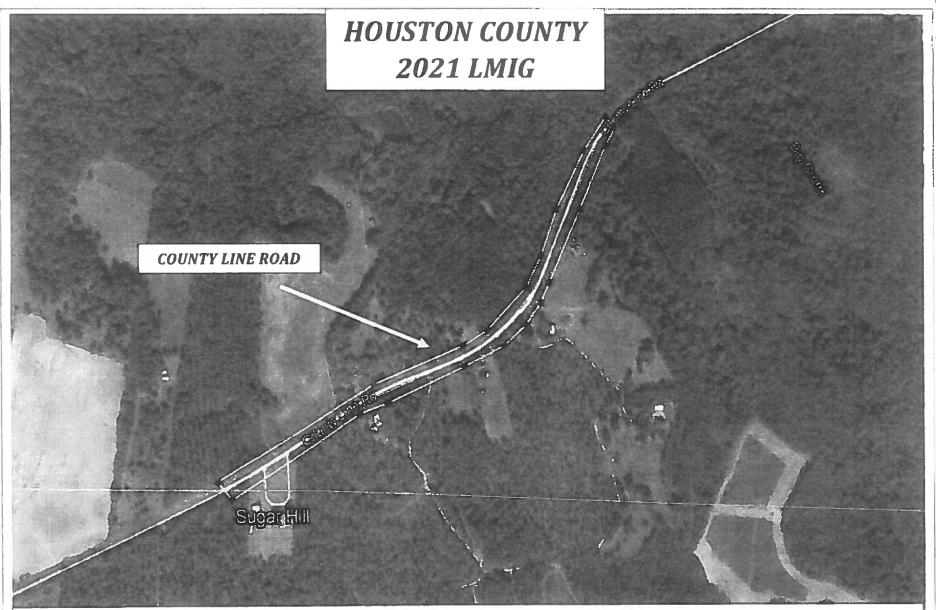
County Line Rd: L=0.75 miles, w=20LF; Begins 0.75 miles West of Loggins Road Intersection and ends at County Line Asphalt: 165LB/SY of 12.5 mm Superpave
